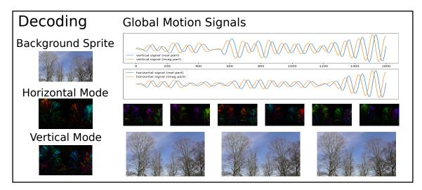
Figure 4: Modal bases are scaled and phase shifted according to the global motion signal, and the background sprite is warped to generate motion.
