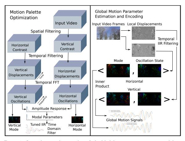
Figure 3: Our video encoding pipeline. Left: Modal parameters are estimated from a short video clip, as described in Section 4. Right: Motion vectors are filtered and projected onto the modal basis to generate global motion parameters as described in Section 5.
